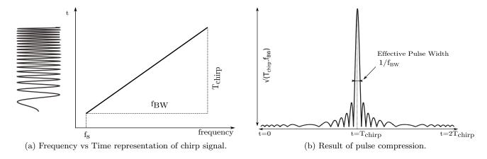
Figure 1: Chirp signals: (a) The linear variation of chirp signal frequency with time. (b) Compressed pulse output of the matched filter.
