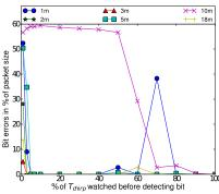
(a) Early detection of chirps on simulated AWGN channel.
