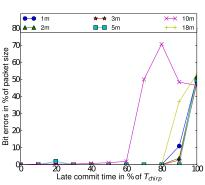
(a) Late commit on chirps with  $T_{chirp}=1\mu\,\mathrm{s}$  and simulated AWGN channel.
