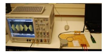
Figure 7: The signal acquisition setup for recording NanoLOC transciever CSS transmissions.
