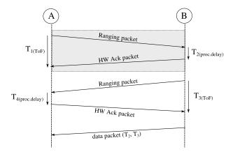
Figure 3: SDS-TWR ranging scheme: RTOF measurements  $(T_{1(ToF)}, T_{3(ToF)})$  are calculated by both nodes A and B. In the final step node B exchanges its time measurements with A. In a single sided two way ranging (highlighted), the RTOF measurement is calculated by node A only.
