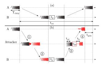
Figure 4: Distance decreasing attack: (a) CSS ranging in a non-adversial setting where  $t_{rtt}$  is the estimated RTOF. (b) Attacker reduces the total round-trip time to  $t_{rtt}-t_{gain}$  by performing early detect and late commit on node B's response CSS signal while communications from A to B are relayed without any LC or ED.
