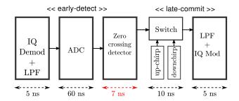
Figure 9: Attacker hardware: The zero crossing detector algorithm tested on a FPGA introduced a delay of 7 ns. Specified time delays of other blocks are based on COTS hardware specifications.
